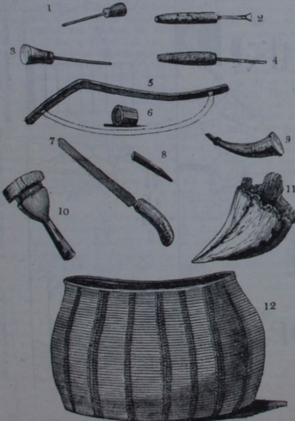
Tools of an Egyptian Carpenter. (Wilkinson.) FIG. 1, 2, 3, 4. Chisels and drills. 5. Part of drill. 6. Nut of wood belonging to drill. 7, 8. Saws. 9. Horn of oil. 10. Mallet. 11. Basket of nails. 12. Basket which held them.
