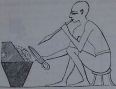
Egyptian Blow-pipe, and small fireplace with cheeks to confine and reflect the heat. (Wilkinson.)
